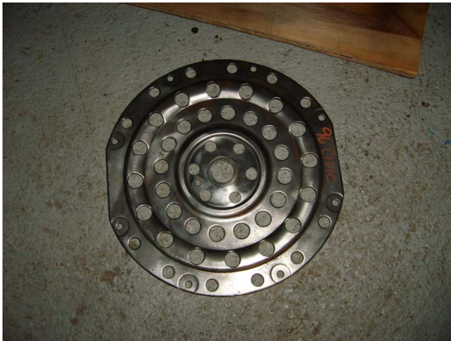
This is the Flex Plate. This connects the engine to the transmission much like a Flywheel from a manual transmission, except this is thinner than a flywheel. It is normally part of the engine and not a transmission so make sure you keep this before you get rid of your engine.
