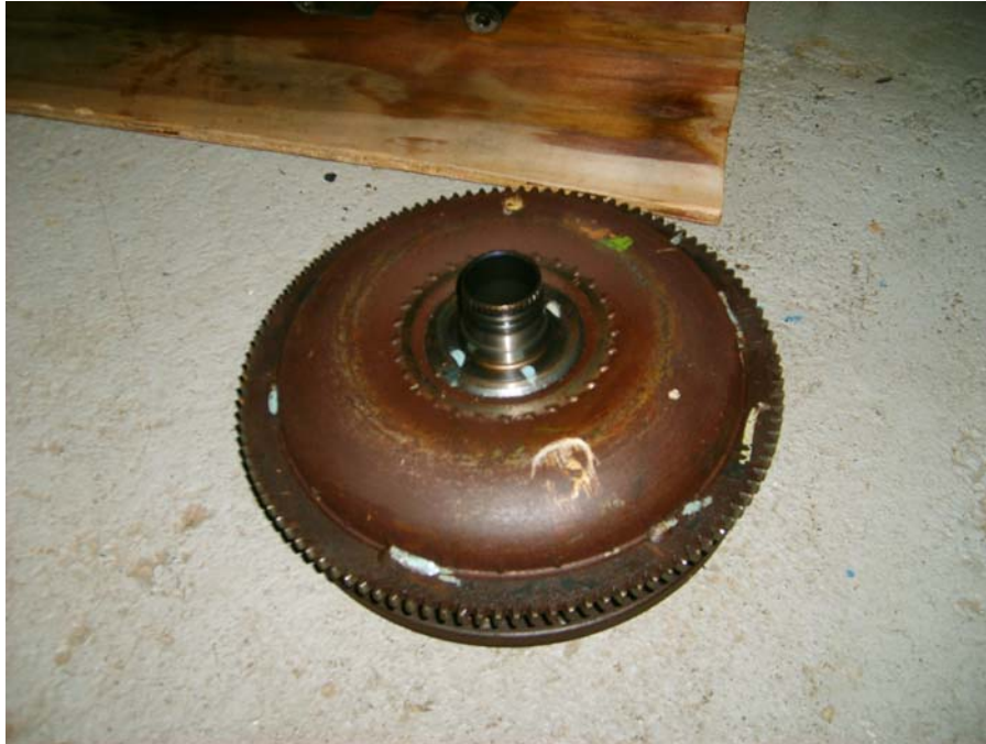
Here is the Torque Converter. This side connects to the shaft on the transmission.
