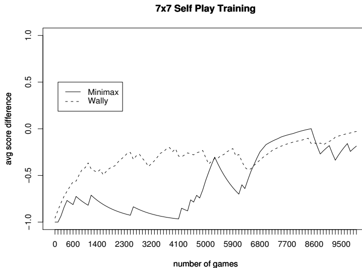
Figure 7.5: Self-play training with softmax in 7x7 games vs. Wally and minimax ( \tau = 0.13 , decaying \alpha , \gamma = 1.0 , \lambda = 0.5 )
