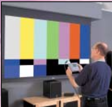
A video generator is used to generate precision test signals.
