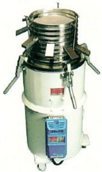
RBF-15 With multi-deck options (10", 12" & 15" Screen Dia.)
